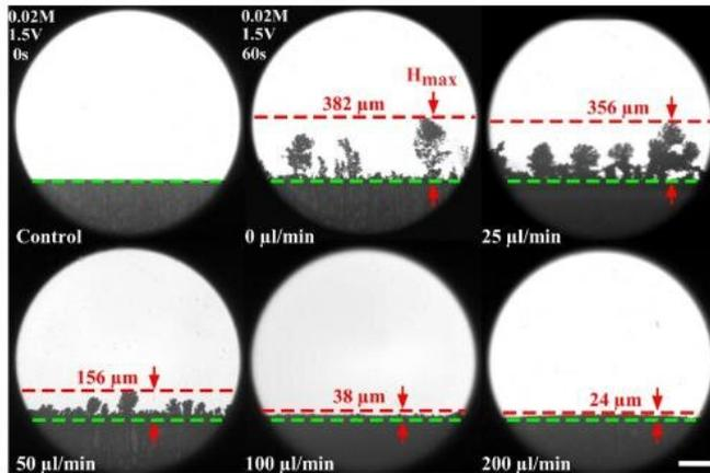
Increasing the flow rate over the electrode reduced the growth of dendrites on the surface. Credit: Jiandi Wan
