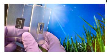
The efficiency of solar cells can be increased by combining two light-absorbing materials. Such tandem devices derive energy from both direct sunlight and light reflected from other surfaces. Credit: KAUST; Anastasia Serin
