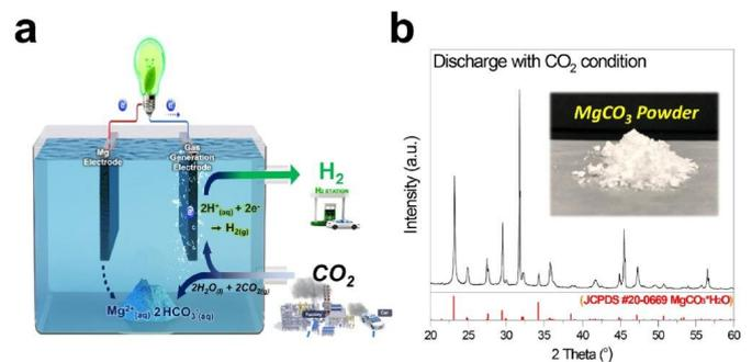
(a) Schematic illustration of MF Mg-CO<sub>2</sub> battery. (b) The XRD profile of the precipitated white solid after discharge process in CO<sub>2</sub> sat'd condition and N<sub>2</sub> sat'd condition. Credit: Ulsan National Institute of Science and Technology
