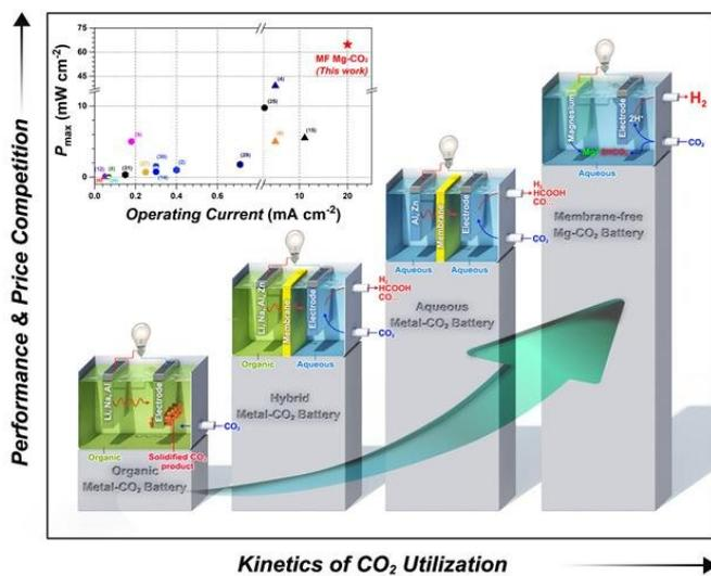
(MF) Mg-CO<sub>2</sub> battery, as an advanced approach to sequester CO<sub>2</sub> emissions by generating [electricity](#) and value-added chemicals without any harmful by-products. According to the research team, their MF Mg-CO<sub>2</sub> battery operates based on the indirect utilization of CO<sub>2</sub> with facile hydrogen generation process. It has been also found that the [new battery](#) exhibits high faradaic efficiency of 92.0%.
