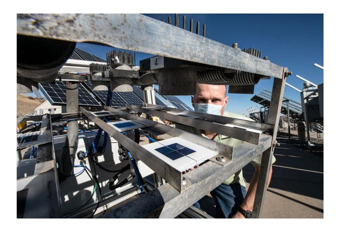
At the Outdoor Test Facility, NREL researcher Matthew Muller looks over the DUSST multi-unit soiling detector. The patented technology has nine individual soiling measurements allowing for comparison of nonuniform soiling and testing of the anti-soiling performance of different glass coatings. Credit: Dennis Schroeder, NREL
