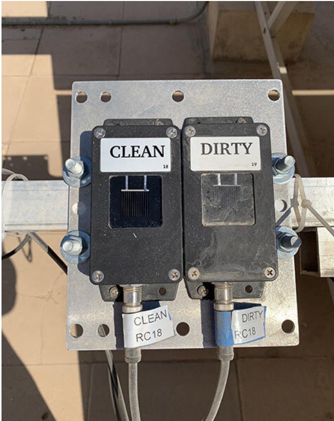
Two sensors in the field show the difference between one that is regularly cleaned and one that never is. Credit: Matthew Muller, NREL
