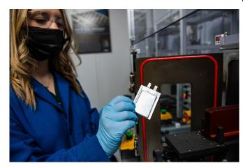
Cassidy Anderson, a PNNL post-bachelor intern and Battery500 Consortium team member, holds a pouch cell battery in PNNL's Advanced Battery Facility. The battery is enclosed in a polymer-based pouch containing an aluminum barrier layer to keep it safely sealed in an air-free environment. Credit: Pacific Northwest National Laboratory.
