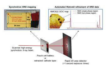
A schematic of the high-energy x-ray powder diffraction setup. Using automated software, the team mapped the battery state of charge (SOC) based on the diffraction data they collected for thousands of points across the battery. Credit: Brookhaven National Laboratory
