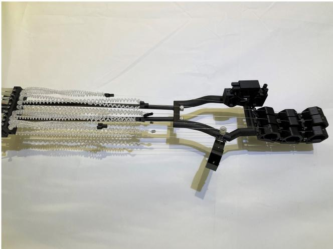
Demonstration of the contraction response and biomimetic application of cavatappi artificial muscles. Credit: Higuera-Ruiz et al., *Sci. Robot.* 6, eabd5383 (2021).
