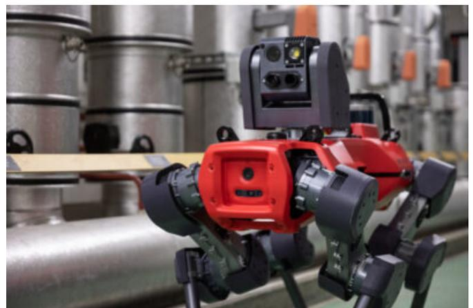
The pan-tilt inspection unit features high-end sensors for accurate and reliable visual, thermal, and acoustic measurements. Credit: ANYbotics
