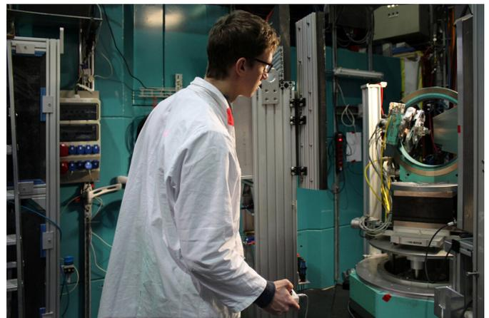
Using the remote control Dr. Tobias Fritsch brings the lattice structure into the correct measuring position in the residual stress diffractometer STRESS-SPEC at the Research Neutron Source Heinz Maier-Leibnitz of the Technical University of Munich. Credit: Dr. Michael Hofmann
