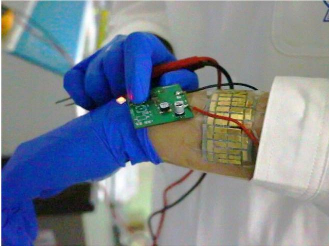
A person wearing the self-powered electric system composed of a TEG band and an LED. Credit: Yijie Liu
