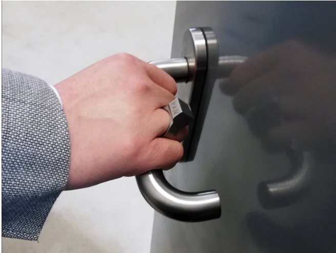
Picture 2: Thanks to the inte-grated RFID tag, the ring produced by the 3D printing process can act as a door opener. Credit: Fraunhofer IGCV
