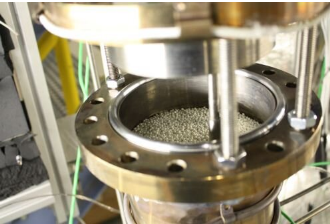
Preliminary test of an electrothermal storage system: A storage system with bulk material and liquid metal as heat transfer fluid. Credit: Franziska Müller-Trefzer, KIT
