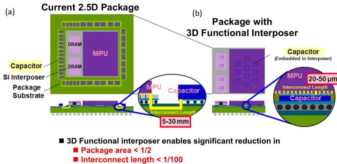
The new interposer design with an embedded capacitor provides a notable reduction in area requirements and interconnect length, leading to lower wiring resistance and parasitic capacitance. MPU: Microprocessing unit; DRAM: Direct random-access memory. Credit: The 2021 IEEE Electronic Components and Technology Conference
