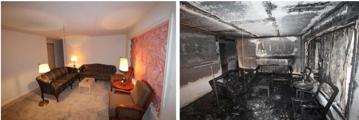
NIST tested P-Flash further by comparing its predicted temperature data to temperatures measured in 13 real house fires, purposefully lit during Underwriters Laboratories (UL) experiments. The aftermath of a UL experiment can be seen in before-and-after photos of the house's living room, along with a temperature sensor strung from the ceiling. Credit: UL Firefighter Safety Research Institute
