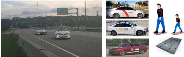
Figure 5: Executing the test cases precisely (a cut-in example is shown on the left) using the Mcity test vehicles
