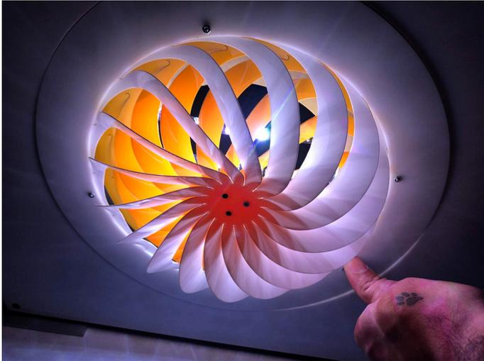
By harnessing the mechanical instabilities in curved beams, researchers developed a system that can transform objects into elaborate and customizable 3D configurations. Above, the researchers demonstrated a lamp shade that can open and close in a simple motion. Credit: Saurabh Mhatre/Harvard University
