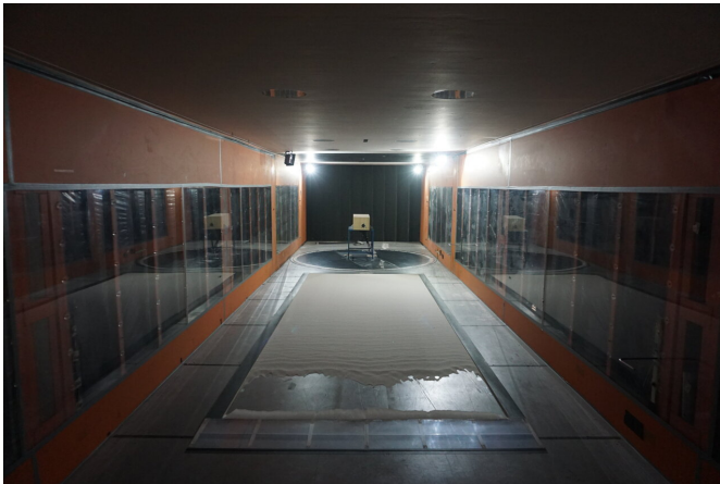
The HyPer SMM team carried out wind tunnel tests to characterise how sand moves at different wind speeds. Credit: Lorenzo Raffaele
