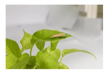
University of California, Berkeley, engineers have created a lightweight and durable robot that achieves exquisite control and agility by modulating the electrostatic forces between its feet and surfaces. Small, robust robots like these could be ideal for conducting search and rescue operations or investigating other hazardous situations, such as scoping out potential gas leaks. Credit: UC Berkeley photo courtesy of Jiaming Liang & Liwei Lin
