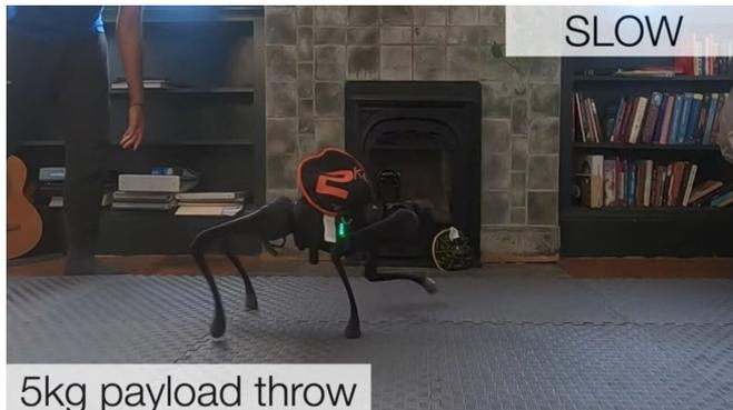
A group of researchers from Carnegie Mellon and UC Berkeley working with a team at Facebook AI has developed a new type of reactive locomotive system for robots. Called rapid motor adaptation, it allows a robot to traverse a variety of terrain types by learning from past experiences. The group has written a paper describing their new technology and how well it worked when tested and have posted it on the arXiv preprint server.
