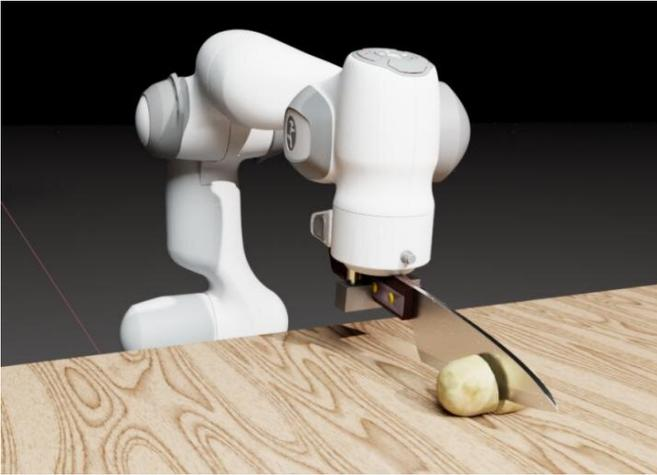
USC PhD student Eric Heiden, working with NVIDIA researchers, has created a new simulator for robotic cutting that can accurately reproduce the forces acting on the knife as it presses and slices through common foodstuffs. Credit: Eric Heiden/NVIDIA
