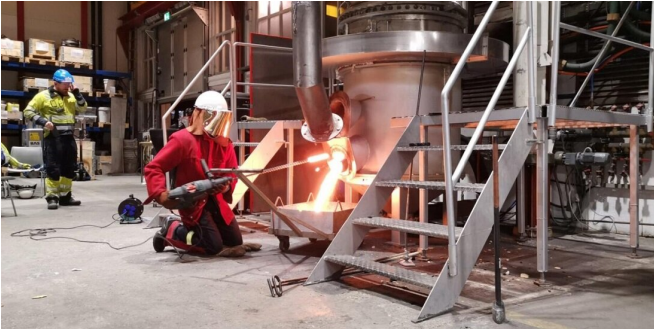
Operators from Elkem Thamshavn are shown tapping liquid silicon from the furnace. Credit: Vegar Andersen
