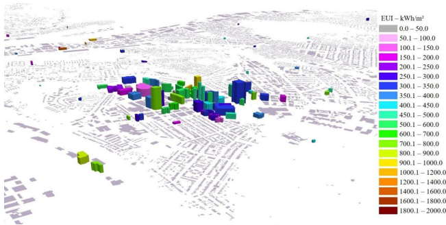
Simulated annual energy use intensity (EUI) of the commercial buildings in the urban building energy model (UBEM) for Pittsburgh, Pennsylvania. Credit: Bilec Built Environment and Sustainable Engineering Group
