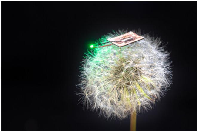
Weighing about as much as two grains of rice but with the energy density of a much larger, heavier battery, the researchers' packaging-free design could enable a host of otherwise impossible electronics. Credit: Penn Engineering Today
