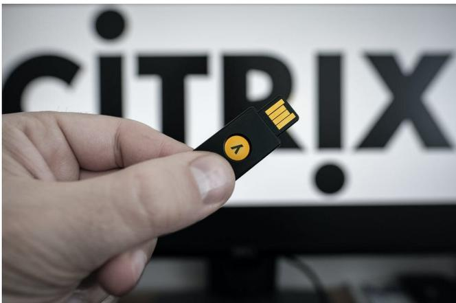
The YubiKey, first developed in 2008, is an authentication device designed to support one-time password and 2FA protocols without having to rely on SMS-based 2FA. Credit: Shutterstock
