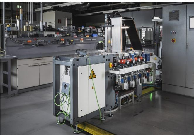
DRYtraec machines do not require long drying tracks and so take up significantly less space than conventional battery electrode manufacturing systems. Credit:
