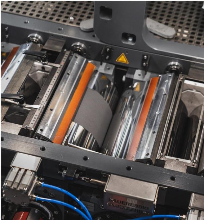
A fine coating film forms on the faster-rotating roller.
