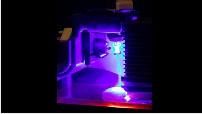
Chicken being cooked by a blue laser. Light is being directed by two software-controlled mirror galvanometers. Credit: Columbia University
