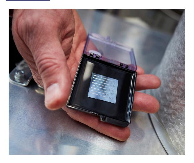
The new component is made of silicon nitride and consists of nine separate waveguides (left). Each waveguide is composed of 22 spirals and can amplify light by about ten times with a noise figure of only 1.2 decibels. Each spiral (right) has an area of 1 square millimeter and the shape enables the compact design of the amplifier. Credit: Henrik Sandsjö/Chalmers University of Technology, Sweden
