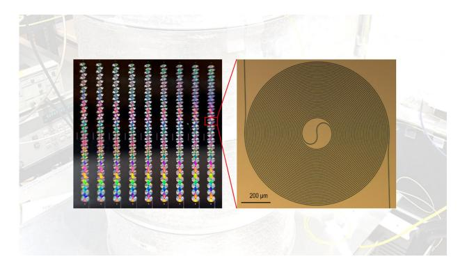
The new component is made of silicon nitride and consists of nine separate waveguides (left). Each waveguide is composed of 22 spirals and can amplify light by about ten times with a noise figure of only 1.2 decibels. Each spiral (right) has an area of 1 square millimeter and the shape enables the compact design of the amplifier. Credit: Zhichao Ye and Yen Strandqvist/Chalmers University of Technology
