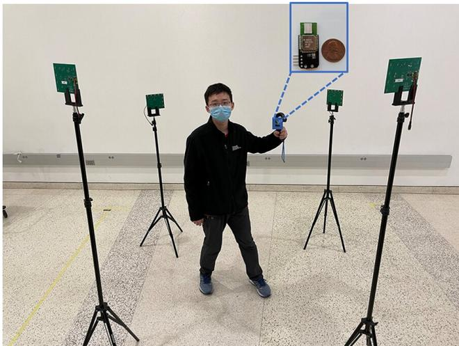
The new UWB system consists of a small electronic tag (inset shows the size of a tag compared to a U.S. penny) that transmits one signal simultaneously to four anchors. Credit: University of California - San Diego
