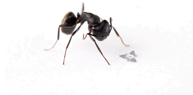
A 3D microflier sits next to a common ant to show scale. Credit: Northwestern University
