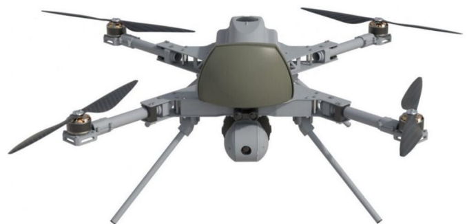
The Kargu-2, made by a Turkish defense contractor, is a cross between a quadcopter drone and a bomb. It has
