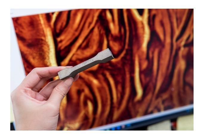
The new titanium alloy developed by City University of Hong Kong using 3D printing has lava-like microstructures that give rise to its excellent mechanical properties. Credit: City University of Hong Kong
