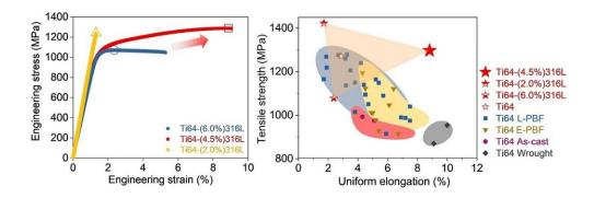
The experimental results show that the new titanium alloy has supreme mechanical properties. Credit: Dr Zhang Tianlong
