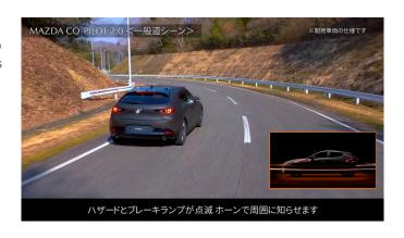
This image provided by Mazda Motor Corp., shows that the Mazda Co-Pilot Concept car flashes hazard lights on and off, after a mock driver has undergone a sudden health problem, and will come to a safe stop, in Miyoshi, Hiroshima prefecture, Japan on Sept. 30, 2021. Vehicles with the Mazda Co-Pilot Concept will warn drivers around them with hazard lamps and horns that the driver has undergone a sudden health problem. Credit: Mazda Motor Corp. via AP
