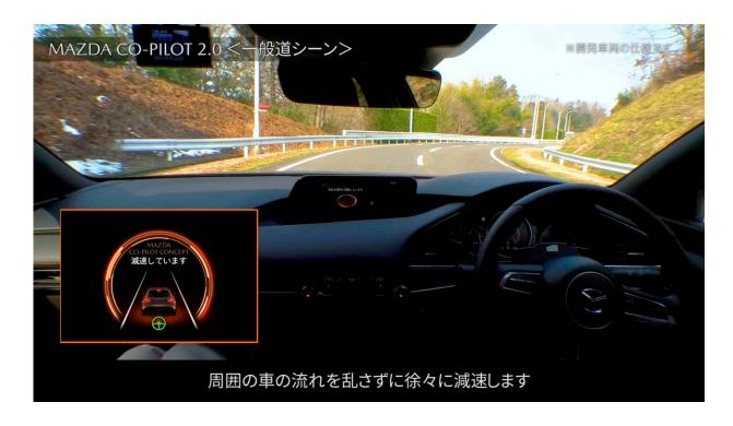
This image provided by Mazda Motor Corp., shows the dashboard of the Mazda Co-Pilot Concept car in Miyoshi, Hiroshima prefecture, Japan on Sept. 30, 2021. Cameras that are part of the Mazda Co-Pilot Concept will know through the image data that the driver has had a sudden health problem. The words at bottom read " (The vehicle) gradually slows down without impeding the flow of traffic." A rendering, left, shows an enlarged monitor on the dashboard. Credit: Mazda Motor Corp. via AP
