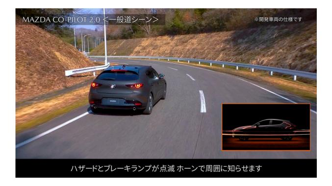
This image provided by Mazda Motor Corp., shows that the Mazda Co-Pilot Concept car flashes hazard lights on and off, after a mock driver has undergone a sudden health problem, and will come to a safe stop, in Miyoshi, Hiroshima prefecture, Japan on Sept. 30, 2021. Vehicles with the Mazda Co-Pilot Concept will warn drivers around them with hazard lamps and horns that the driver has undergone a sudden health problem. Credit: Mazda Motor Corp. via AP
