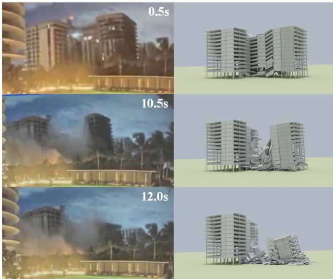
Comparison between actual and simulated collapse process. Credit: Andy Slater
