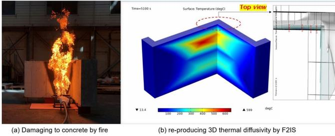
With information of time-temperature curves resulted from DIA, 3D thermal diffusivity is re-produced. Commercial program of 'Comsol Mutiphysics' is used for this simulation work. Location of fire source and thermal spread are traced without pre-installed sensors after fire exposure. Credit: Korea Institute of Civil Engineering and Building Technology (KICT)
