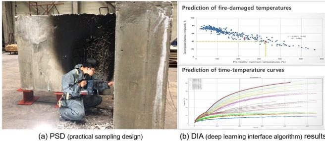
(a) With a portable hand drilling device, samples of only 1~2 g are being taken at every 10 mm depth, up to 40 mm so that the least damage to the concrete specimen is achieved. (b) Final outputs of fire-damaged temperatures at each depth where samples are taken and time-temperature curves at surface of the concrete specimen are resulted from computational work of DIA. Credit: Korea Institute of Civil Engineering and Building Technology (KICT)
