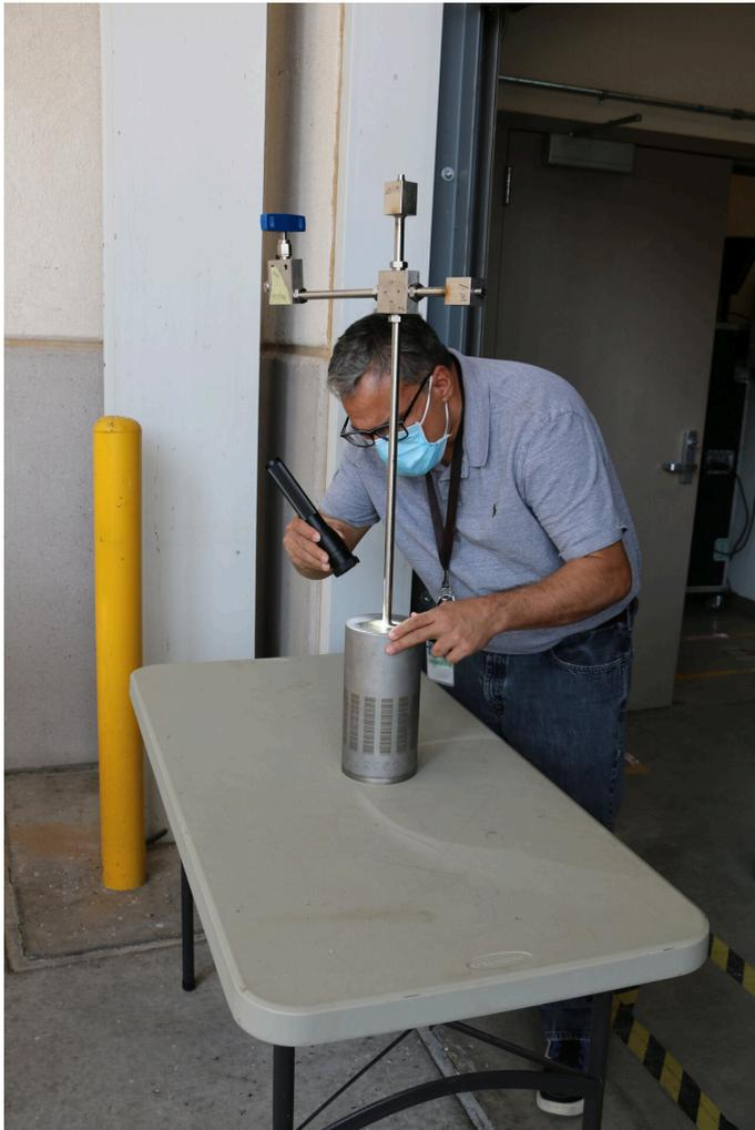
Victor Figueroa, a Sandia National Laboratories quality-assurance coordinator, inspects a specially designed stainless-steel container prior to heating it to 2000 degrees Fahrenheit to ensure the safety of the container for the storage and transportation of hazardous materials. Credit: Sandia National Laboratories
