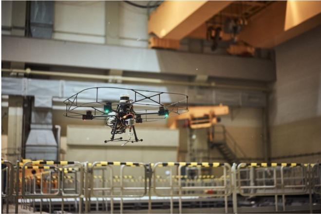
A drone using autonomy software developed by Southwest Research Institute navigated an inoperable nuclear facility, during the October 2021 EnRich hackathon. Using LIDAR data and exploration algorithms, SwRI built a map of the test facility by simultaneously localizing and mapping the environment. Credit: SwRI
