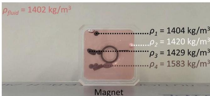
Height differences of plastic particles inside a ferrofluid. Credit: Eindhoven University of Technology
