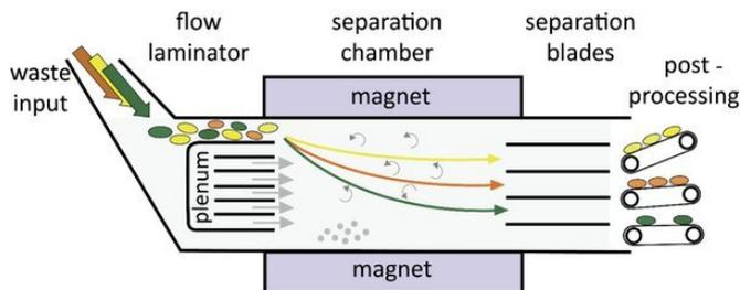
Schematic of the separation process. Credit: Eindhoven University of Technology
