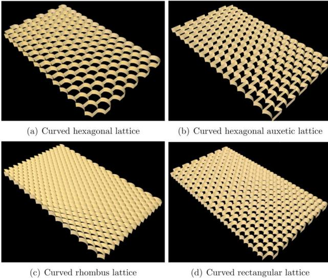
Family of curved 2D lattices conceived and analyzed in the study (a) The curved hexagonal lattice, (b) The curved hexagonal auxetic lattice, (c) The curved rhombus lattice, and (d) The curved rectangular lattice. Credit: S. Mukherjee
