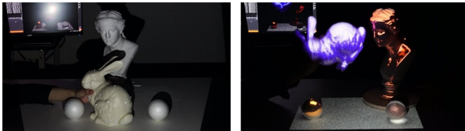
Figure 1. Recently developed projection mapping techniques can achieve a very realistic appearance, even in dynamic scenes. However, they suffer from critical limitations, such as the need for markers on moving projection targets. In the above photographs, the markers can be clearly seen on the bunny. Credit: Yoshihiro Watanabe from Tokyo Tech
