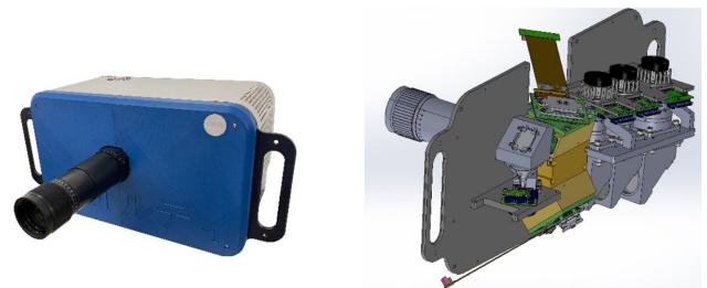
Figure 2. The developed projector has a unique optics engine (shown on the right) and two digital micromirror devices that enable it to project RGB and IR images with excellent alignment accuracy. Credit: Yoshihiro Watanabe from Tokyo Tech and the source and copyright of ITE and SID
