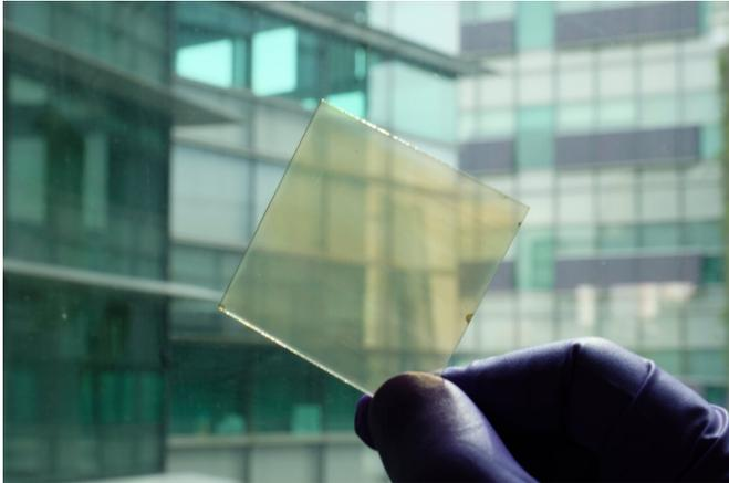
The self-adaptive glass developed by NTU Singapore scientists has a unique structure that modulates heating and cooling simultaneously. Credit: NTU Singapore
