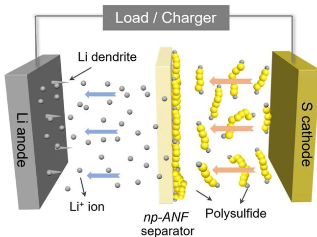
A diagram of the battery shows how lithium ions can return to the lithium electrode while the lithium polysulfides can't get through the membrane separating the electrodes. In addition, spiky dendrites growing from the lithium electrode can't short the battery by piercing the membrane and reaching the sulfur electrode. Credit: Ahmet Emre, Kotov Lab
