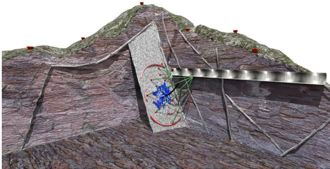
GeoLaB is a generic geoscientific underground laboratory in crystalline bedrock. Research is aimed at a safe and ecologically sustainable use of major geothermal energy resources in Germany. Credit: KIT
