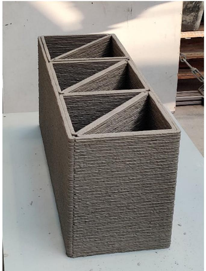
A building envelope prefabricated using the 3D printing process. Credit: Mehdi Chougan, Author provided
