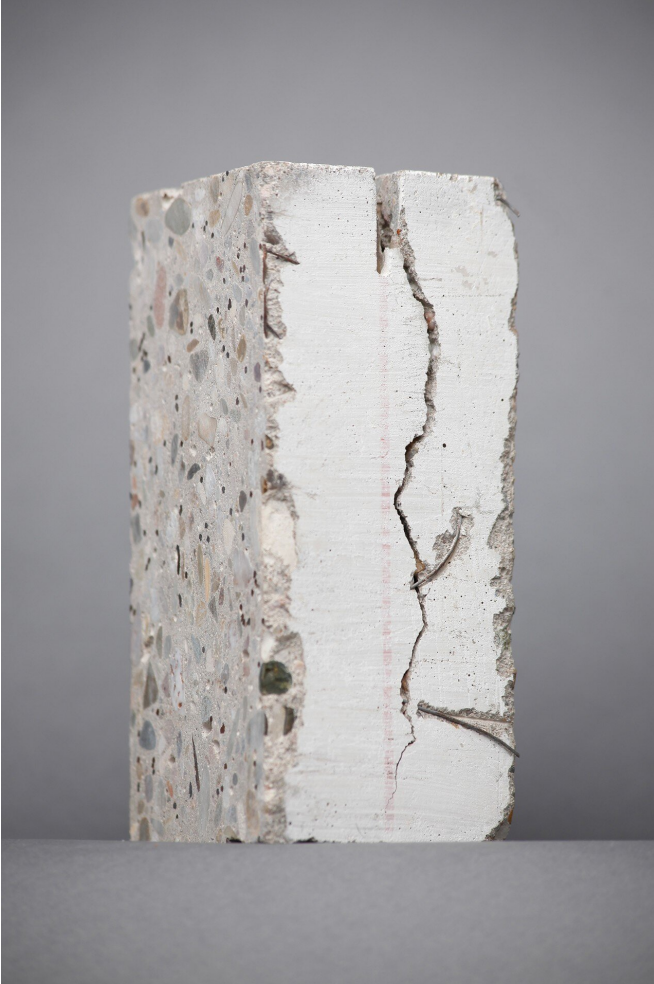
Concrete sample with crack. Credit: Fraunhofer-Gesellschaft
