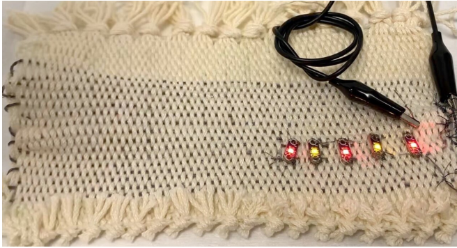
Supercapacitor yarns integrated in a fabric for powering LEDs. Credit: Nanfei He
