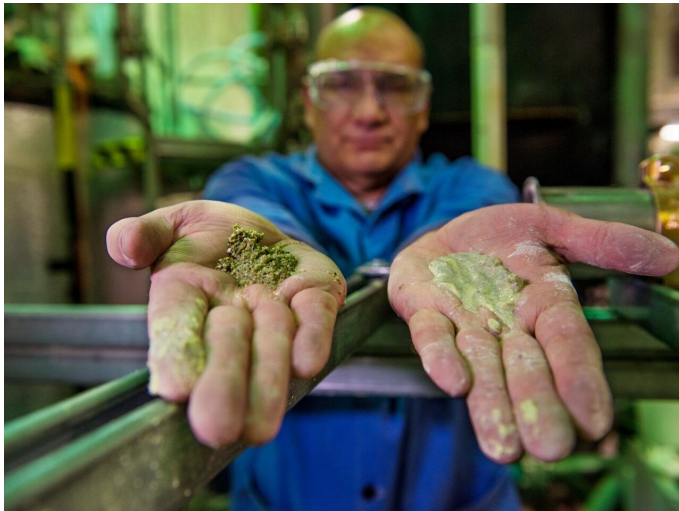
Michael Minette shows 300-micron and larger particles separated out of a slurry mixture using Pacific Northwest National Laboratory's mesofluidic separator. These results came from tests on simulant at PNNL's Multi-Phase Transport Evaluation Laboratory. Credit: Andrea Starr | Pacific Northwest National Laboratory
