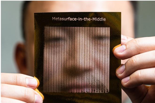
Rice University graduate student Zhambyl Shaikhanov holds a foil sheet he used to create a "metasurface"—a paper sheet covered with a 2D foil pattern—that an eavesdropper could use in a "Metasurface-in-the-Middle" attack to redirect part of a high-frequency "pencil beam" transmission like those planned for 6G wireless networks. Credit: Jeff Fitlow/Rice University
