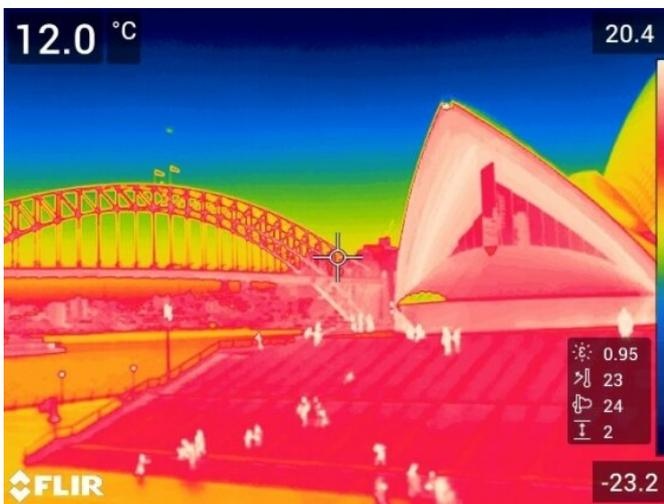
A thermal imaging camera highlights the amount of heat radiating from Sydney Harbour and its surroundings back into the atmosphere at night. Credit: University of New South Wales
