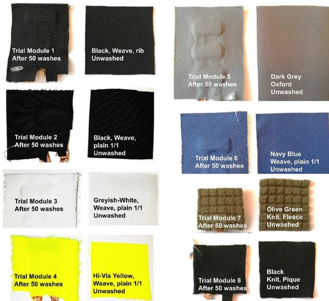
Textile solar modules before (right) and after 50 cycles of washing (left). Credit: *Research Journal of Textile and Apparel* (2022). DOI: 10.1108/RJTA-01-2022-0004
