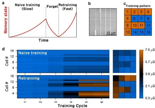
Retraining operation in the neuromorphic device array. a) Schematic graph showing the retraining effect. b) Scanning electron microscope image of the neuromorphic device array. c) Training pattern “F” for the retraining test. d) Evolution of the memory state of the neuromorphic device array for the naive training and retraining scheme. Credit: The Korea Advanced Institute of Science and Technology (KAIST)
