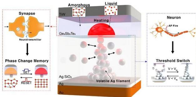
Neuromorphic memory device consisting of bottom volatile and top nonvolatile memory layers emulating neuronal and synaptic properties, respectively. Credit: The Korea Advanced Institute of Science and Technology (KAIST)
