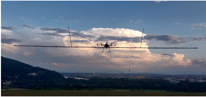
Airborne Optical Sectioning (AOS) drone prototype for real-time through-foliage tracking of moving targets. Credit: Journal of Remote Sensing
